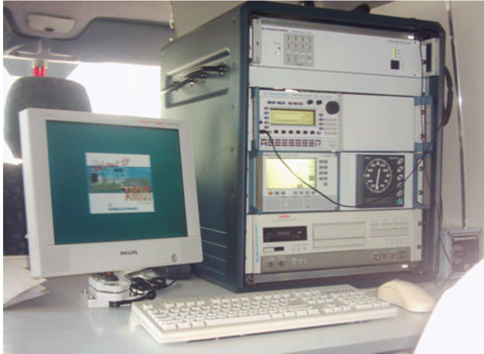
Figure 05: The internal view of the frequency-monitoring vehicle.
