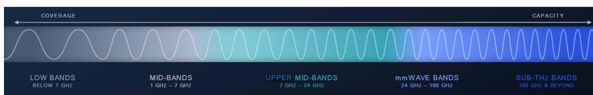
Fig. 1: Low, Mid and High 5G frequency bands
